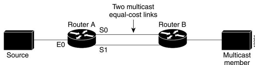
If a tunnel is configured between Router A and Router B, and multicast traffic is made to reverse path forward over the tunnel, then the multicast packets are sent encapsulated into the tunnel as unicast packets between Router A and Router B. The underlying unicast mechanism will then perform load splitting across the equal-cost links.
