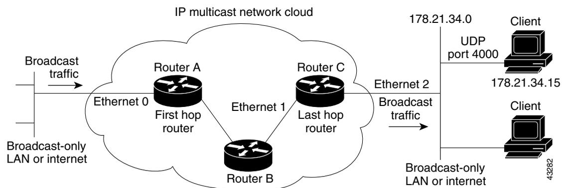
The configuration on the first hop router converts a broadcast stream arriving at incoming Ethernet interface 0 destined for UDP port 4000 to a multicast stream. The access list denies other traffic from being forwarded into the multicast cloud. The traffic is sent to group address 224.5.5.5. Because fast switching does not perform such a conversion, the **ip forward-protocol** global configuration command causes the proper process level to perform the conversion.
