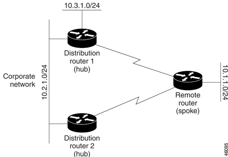
[Figure 50](#) shows a simple dual-homed remote router where distribution router 1 is connected to both network 10.3.1.0/24 and network 10.2.1.0/24.
