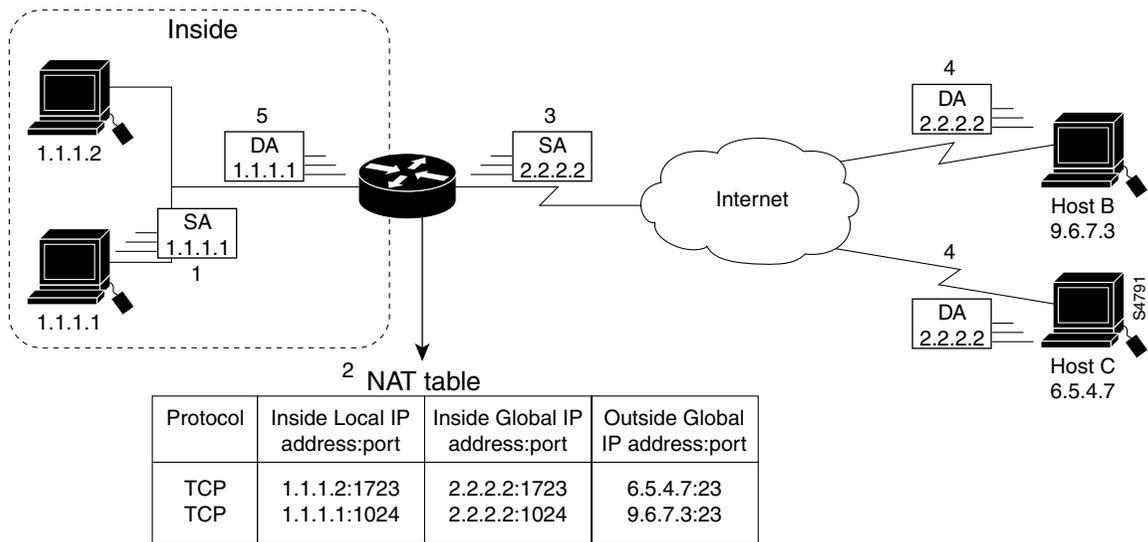
The router performs the following process in overloading inside global addresses, as shown in Figure 5. Both host B and host C believe they are communicating with a single host at address 2.2.2.2. They are actually communicating with different hosts; the port number is the differentiator. In fact, many inside hosts could share the inside global IP address by using many port numbers.
