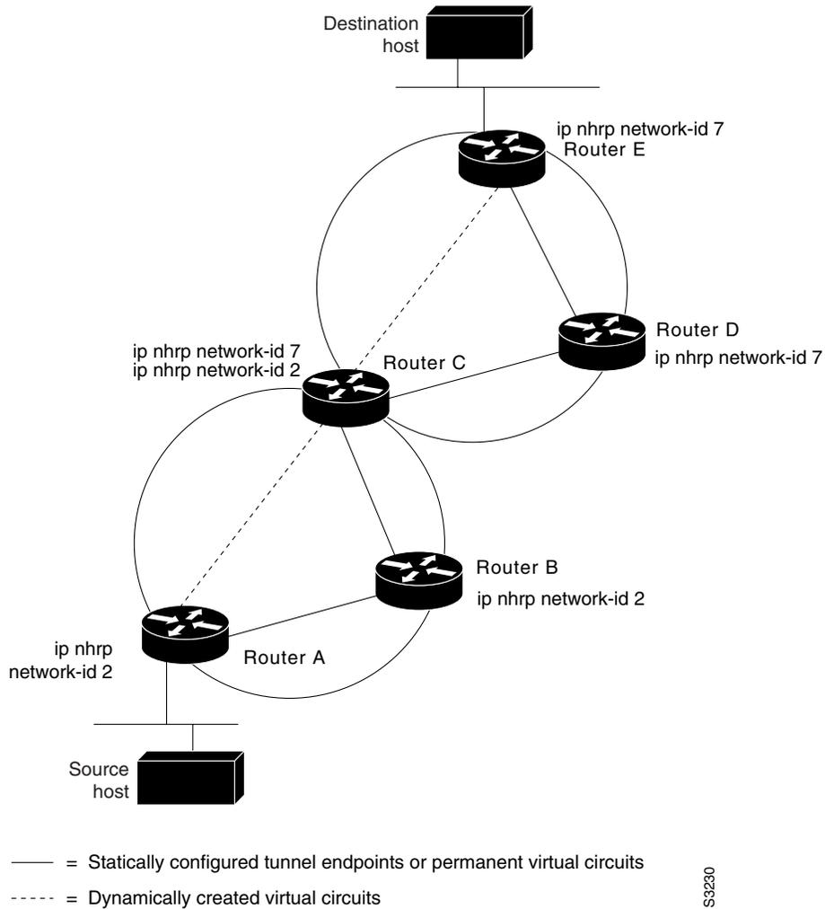
The physical configuration of the five routers in [Figure 9](#) might actually be that shown in [Figure 10](#). The source host is connected to Router A and the destination host is connected to Router E. The same switch serves all five routers, making one physical NBMA network.
