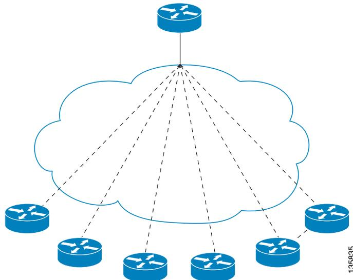
These stub networks might consist only of end systems and the stub router, and thus do not require the stub router to learn any dynamic IP routing information.
