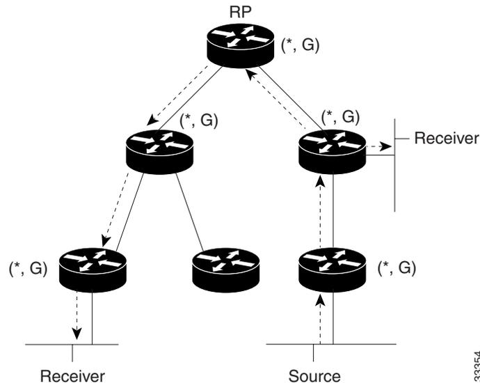
When packets are forwarded downstream from the RP toward receivers, there are no fundamental differences between bidir-PIM and PIM-SM. Bidir-PIM deviates substantially from PIM-SM when passing traffic from sources upstream toward the RP.
