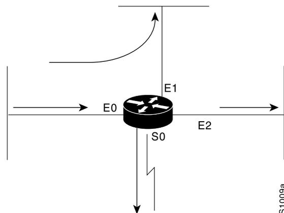
A directed broadcast address includes the network or subnet fields. For example, if the network address is 128.1.0.0, the address 128.1.255.255 indicates all hosts on network 128.1.0.0, which would be a directed broadcast. If network 128.1.0.0 has a subnet mask of 255.255.255.0 (the third octet is the subnet field), the address 128.1.5.255 specifies all hosts on subnet 5 of network 128.1.0.0—another directed broadcast.
