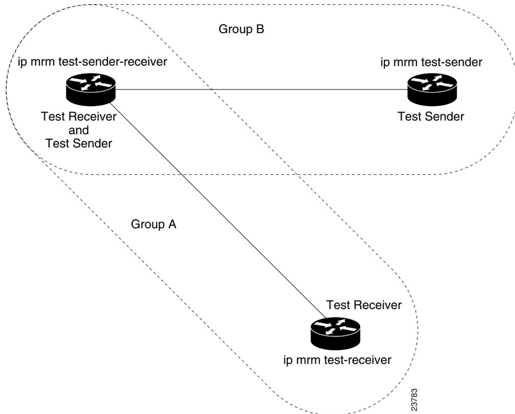
To configure the routers in Figure 86 for monitoring more than one multicast group, configure the Test Sender in Group B and the Test Receiver in Group A separately, as already discussed, and configure the following commands beginning in global configuration mode on the router or host that belongs to both Group A and Group B (in the upper left of Figure 86):
