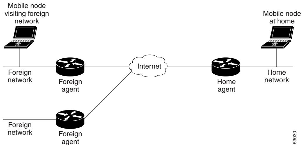
An MN is a node, for example, a PDA, a laptop computer, or a data-ready cellular phone, that can change its point of attachment from one network or subnet to another. This node can maintain ongoing communications while using only its home IP address.
