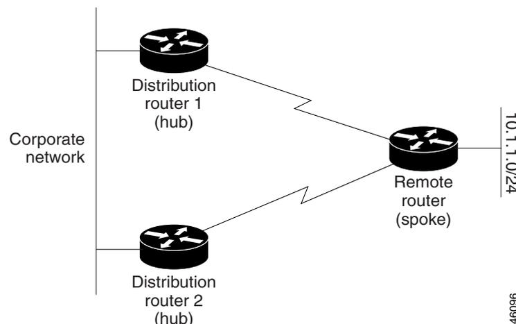
[Figure 49](#) shows a simple dual-homed remote with one remote router and two distribution routers. Both distribution routers maintain routes to the corporate network and stub network 10.1.1.0/24.
