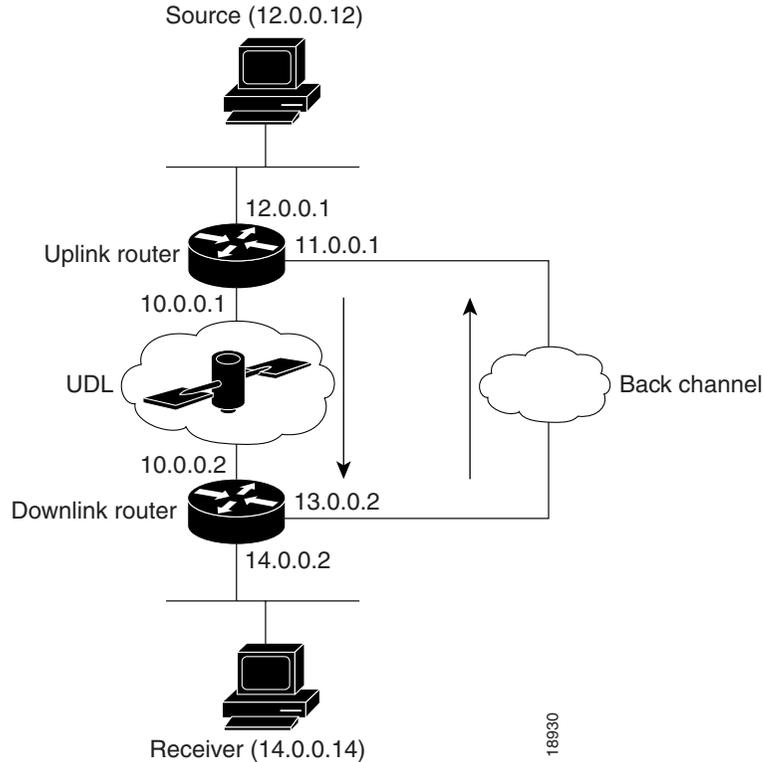
**Uplink Router (uplink-rtr) Configuration**
