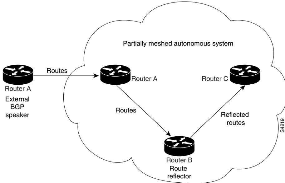
The internal peers of the route reflector are divided into two groups: client peers and all the other routers in the autonomous system (nonclient peers). A route reflector reflects routes between these two groups. The route reflector and its client peers form a *cluster*. The nonclient peers must be fully meshed with each other, but the client peers need not be fully meshed. The clients in the cluster do not communicate with iBGP speakers outside their cluster.
