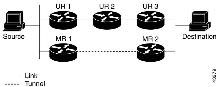
To make the configuration in Figure 69 work, MR 1 and MR 2 must run another routing protocol (typically a different instantiation of the same protocol running in the UR routers), so that paths from sources are learned dynamically.
