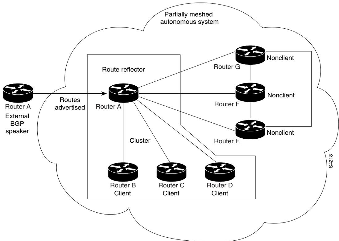
Figure 57 illustrates a more complex route reflector scheme. Router A is the route reflector in a cluster with routers B, C, and D. Routers E, F, and G are fully meshed, nonclient routers.
