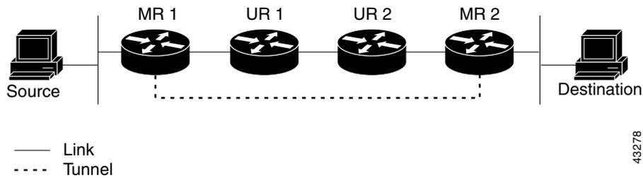
In Figure 68, Source delivers multicast packets to Destination by using MR 1 and MR 2. MR 2 accepts the multicast packet only if it believes it can reach Source over the tunnel. If this situation is true, when Destination sends unicast packets to Source, MR 2 sends them over the tunnel. Sending the packet over the tunnel could be slower than natively sending the it through UR 2, UR 1, and MR 1.
