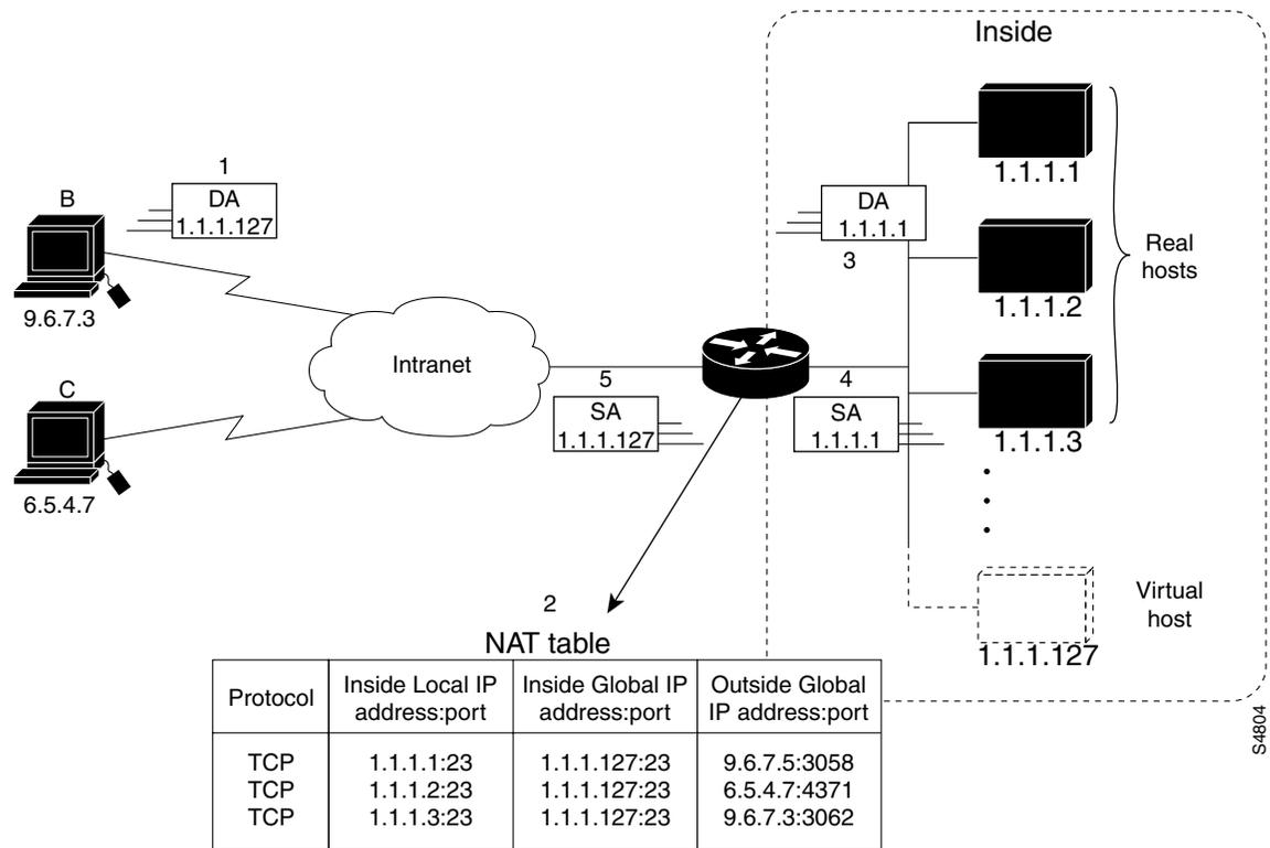
The router performs the following process when translating rotary addresses:
