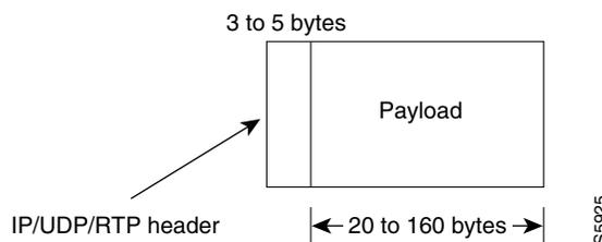
The RTP header compression feature compresses the IP/UDP/RTP header in an RTP data packet from 40 bytes to approximately 2 to 5 bytes, as shown in [Figure 70](#). It is a hop-by-hop compression scheme similar to RFC 1144 for TCP/IP header compression. Using RTP header compression can benefit both telephony voice and MBONE applications running over slow links.
